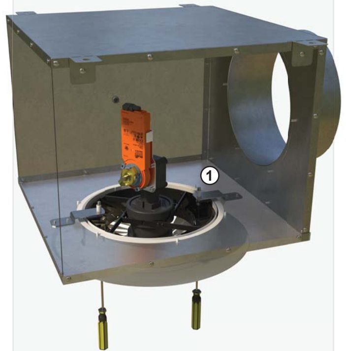
Figure 4 - Installation of an HSC-AD (shown with electric adjustment) into a plenum box using 2pcs M6 bolts ① accessible through the diffuser face. Suitable for sizes DN250-DN500 with electric, thermal or manual adjustment.
