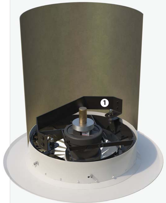
Figure 6 - Installation of an HSC-AD (shown with thermal element) into a round duct with mounting bracket ① using 2pcs M6 bolts accessible through the diffuser face. Suitable for sizes DN250-DN500 with electric, thermal or manual adjustment.
