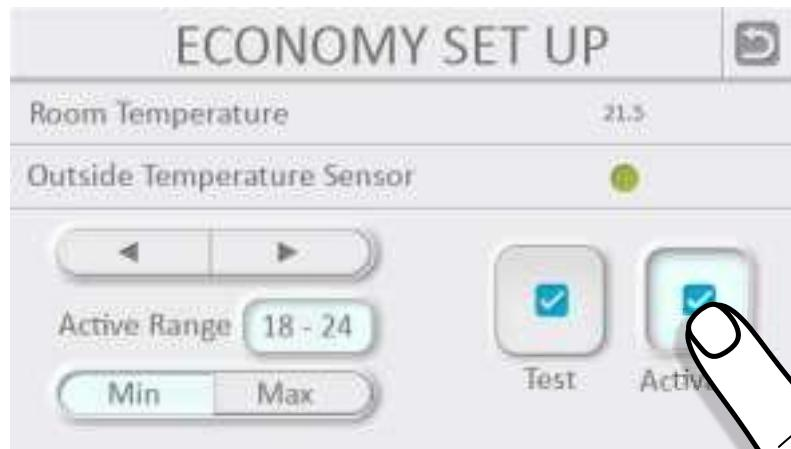
So when the system is in Cooling Mode, if the measured outside air drops to less than Room Temperature (provided this is within the adjustable Active Range) for a continuous period of 5 minutes, the Economy Mode is activated and will be indicated by an 'E' icon in the top left corner of the Base Screen.
