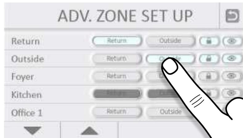
NOTE: Zones set as 'Return' or 'Outside' air are automatically locked and hidden on the Base Screen.
