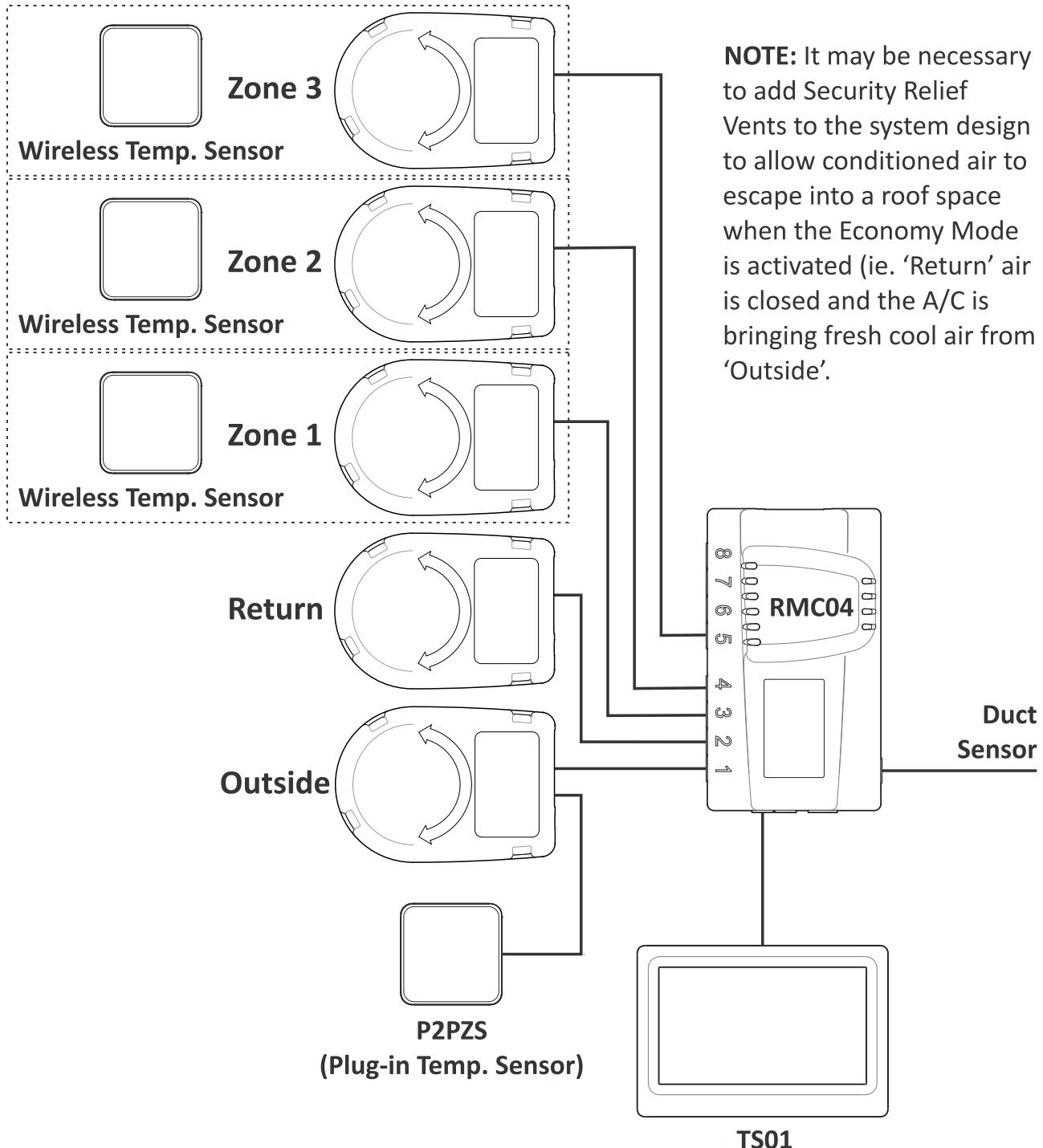
**NOTE:** The Plug-in Temperature Sensor should be mounted in outdoor shade so a reasonable measurement of outside temperature can be obtained. If more than one Zone is configured for 'Outside' air, it doesn't matter which of these Zone Dampers the Sensor is linked to.
