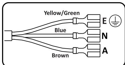
Ensure QC terminals are matched up correctly and fully engaged
